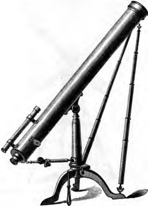
TELESCOPE MOUNTED ON A PILLAR-AND-CLAW STAND, WITH FINDER, VERTICAL AND HORIZONTAL RACK MOTIONS, AND STEADYING RODS.
